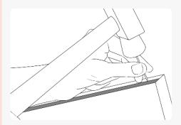
Step 7 Check that no nails, screws or other obstructions that may damage the door are protruding into the cavity.
