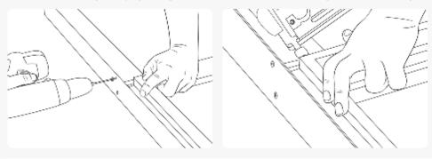
Step 3 Fix the closing jamb to the head section, fixing through the closing jamb into timber reveal. **Note:** No closing jamb provided with plaster reveal units.
