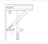
Step 3 Insert the front spear into the bracket as shown in Diagram 3 and fix off. Adjust bolts to ensure the door closes flush to jamb.
