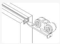
Position rear roller in the hole closest to the edge of door.
