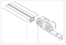
Position leading roller in the hole furthest from edge of door.
