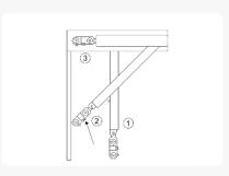
Angle the door into the cavity. Slip the rear roller bolt into the slot of the Fast Fix bracket. The door will easily clip into place. Repeat this process for the front roller. Adjust the bolts to ensure the door closes flush to the closing jamb.
