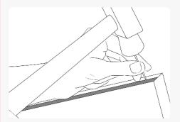
Step 8 Check that no nails, screws or other obstructions that may damage the door are protruding into the cavity.
